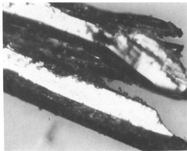
Figure 9 Needle showing the jagged end ( \times 125 ).
